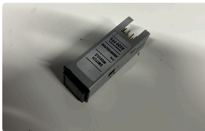
AFTER Finished Simura switch module, produced for A320 FFS installation.
