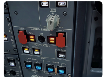
A320 FFS overhead panel pushbuttons.
