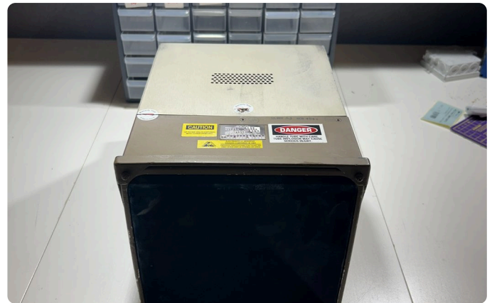
AFTER Reassembled DU-7000, returned for installation-level testing.
