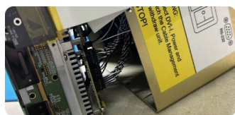
SDU opened: DVI, power and RS-232 interfaces.
